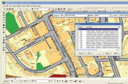
Results from a LocatorHub search. A match ranking is provided with every search result, making it easier for the user to identify the closest matching address.
