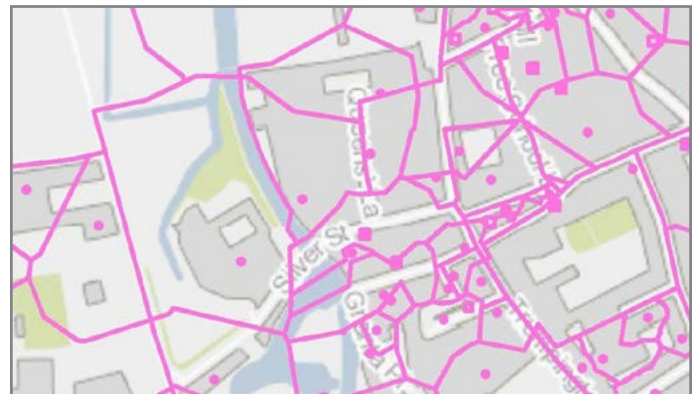
Geoplan XT postcode unit boundaries and GeopointXT overlaid against OS Open 'Background' mapping
